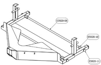
STEP# 2: Insert threaded rods, (E5920-08) through the base supports & crumpler base securing with threaded coupling nuts (E5920-10) & cap nuts (E5920-11).
