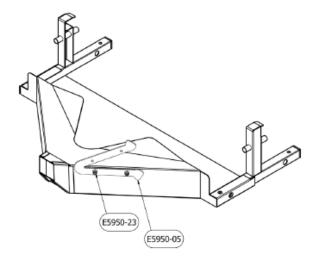
STEP# 3: Attach the "V-Cutter" (E5950-05) to the unit with two nylock nuts, (E5920-23).
