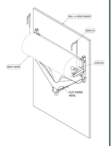
DO NOT OPERATE WITHOUT ROLL COSTRAINT RODS, PART#: E5955-24 in place.
