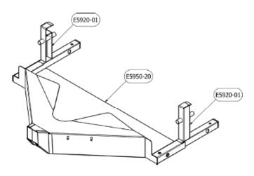
STEP# 1: Slide base support stands, (E5920-01) into the crumpler base. (E5950-20)
