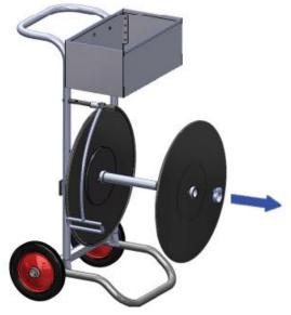
Make sure the unit is standing upright. Release the clamp and remove the front disk.
