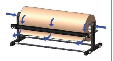
Mount the **center support** back onto the **T-stands**, ensuring that the kraft paper feeds underneath (not over!) the **paper strip**.
