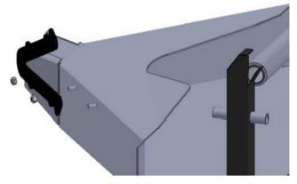
Attach the **paper cutter** to the **base frame** using the included fasteners.
