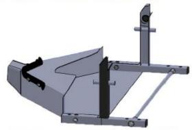
Attach T-Stands to base frame of the EP-5950.
