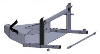
Stabilize **base frame** by attaching the **threaded rod** to the **T-stand**.
