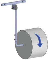
The packaging roll should rotate freely on the Roll Arm. The EP-6000S is now ready for use.
