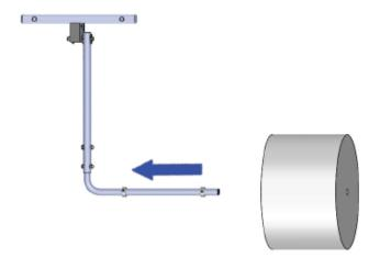
Slide the packaging rolls onto the roll arm.
