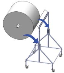
Slide the packaging roll onto the **support** arm.
