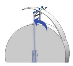
Thread the packaging material under the **brake arm** but over the **cutting arm**. Cut to desired length.
