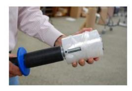
Step One: Untighten the wing so that the stretch film can slide on.
