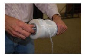
**Step Three:** Tighten the wing so that the rubber expands, to hold the stretch film in place.
